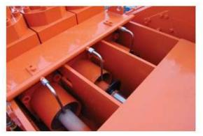
There is also usually a valve on the inlet of the spray bar. This valve should be closed enough so that liner wash fluid does not spray all over the top of the pump and other components.
