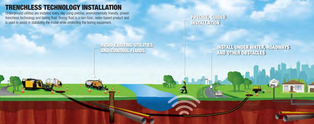
**Trenchless installation equipment** is used to tunnel underground and install utilities with minimal ground disturbance. Trenchless installation is a proven method that has existed for over half a century. It is environmentally friendly and offers a lower carbon footprint than other installation methods. It also produces less noise pollution.
